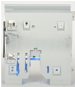
After printing 244,325 pages, the paper path from the printer using only genuine Lexmark Unison Toner was relatively clean, with very little toner spillage visible.
