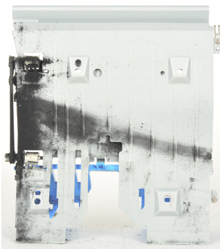
After printing 96,895 pages, the paper path from the printer using Brand #1 cartridges shows moderate toner leakage on one side and mild leakage on the other side.
