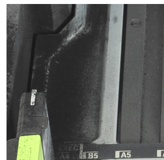
The printer using Brand #4 cartridges shows heavy toner leakage inside the paper drawer.
