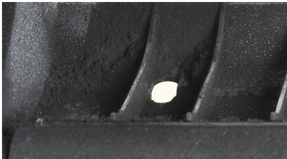
The printer using Brand #1 cartridges shows moderate to heavy toner build-up across the paper feed guide.
