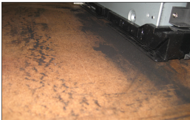
Halfway through BLI's testing, the machine dedicated to Brand #4 toner cartridges showed excessive toner spillage on the desktop around the device. Other third-party brands showed similar toner leakage during testing.
