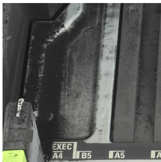
The printer using Brand #1 cartridges shows heavy toner leakage inside the paper drawer.
